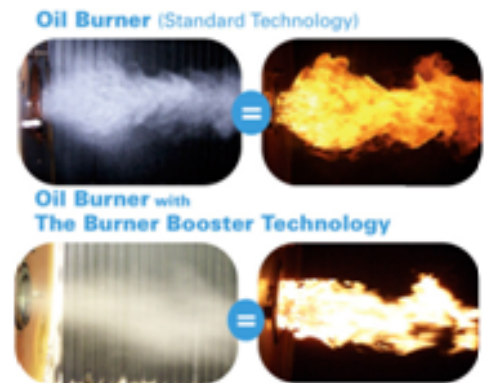
Figure 1. Comparison of tradition burner and Burner Booster combustion.
